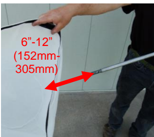
LIGHTLY CLEAN WITH COMPRESSED AIR ONLY, FROM THE OUTSIDE IN. KEEP THE NOZZLE 6-12 INCHES FROM FABRIC
