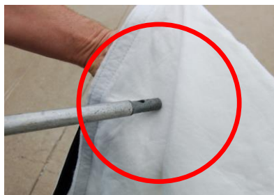
LIGHTLY CLEAN WITH COMPRESSED AIR ONLY, FROM THE OUTSIDE IN. KEEP THE NOZZLE 6-12 INCHES FROM FABRIC
